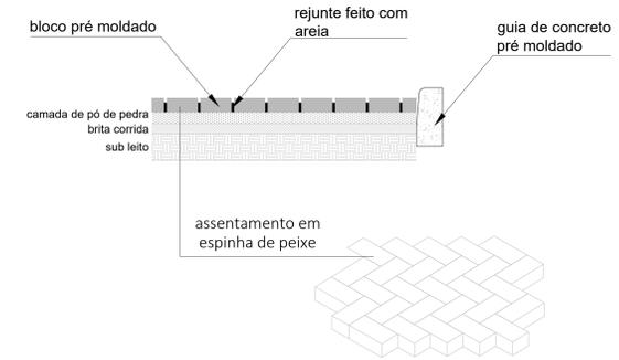
PISTA DE CAMINHADA - DETALHE BLOCO INTERTRAVADO SEM ESCALA
