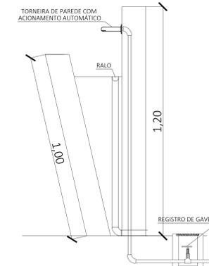
PONTO DE APOIO - DETALHE BEBEDOURO
